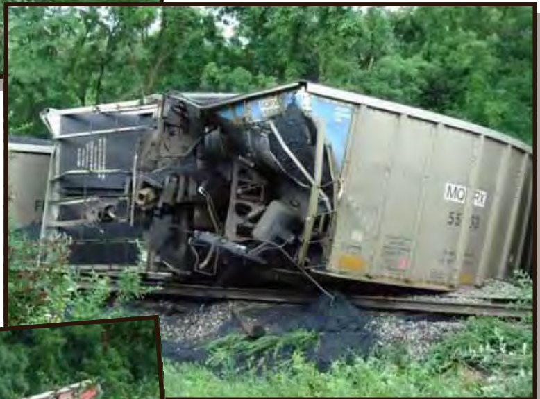
Flood damage to BNSF railroad tracks caused a train derailment in Hanover Township near Hanover
