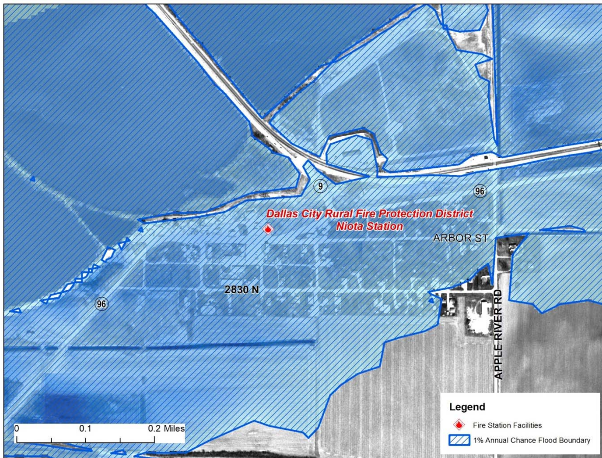
Figure 57: 1% Annual Chance Flood Boundary and Essential Facilities at Risk
