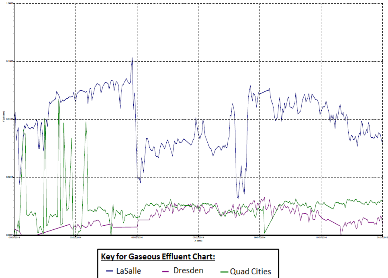
Figure 2. Gaseous Effluent Particulate and Iodine Release Rates from Illinois Nuclear Plants in 2014
